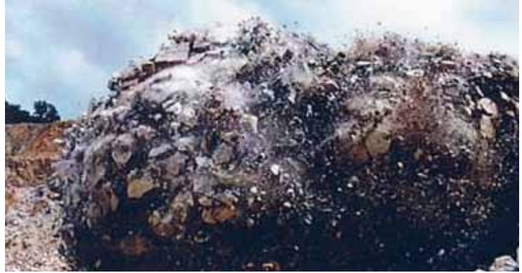
Fig. 4.1. Typical blast at a hard-rock quarry
