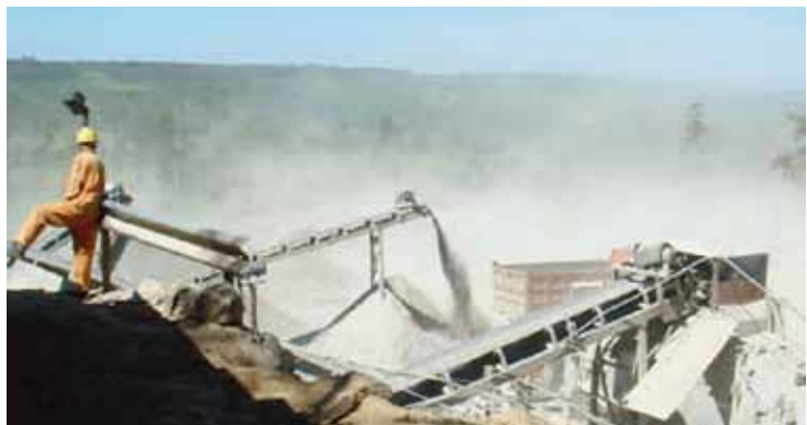
Fig. 3.2. Pre-dust suppression, Kirima Quarry
